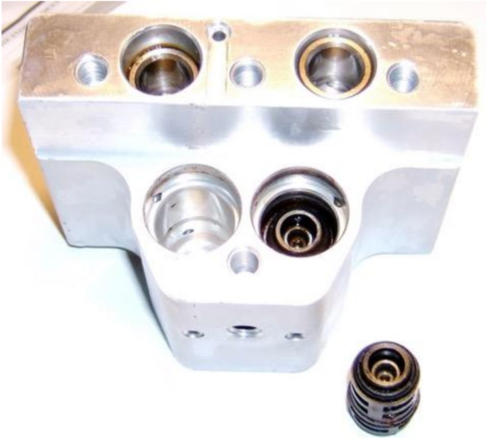
Another wash and clean the solenoid bore, looks better
