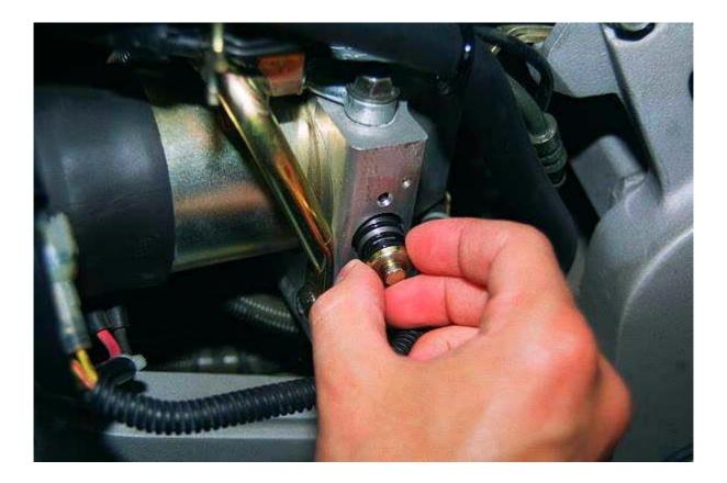
5) Slowly remove the 12mm bolts and the aluminum plate on bottom of the aluminum housing, exposing the buffer chambers. DO NOT remove the rubber plugs. The springs and pistons are the same--the holes they are mounted in are different depths--the deeper is for the front brake circuit.
