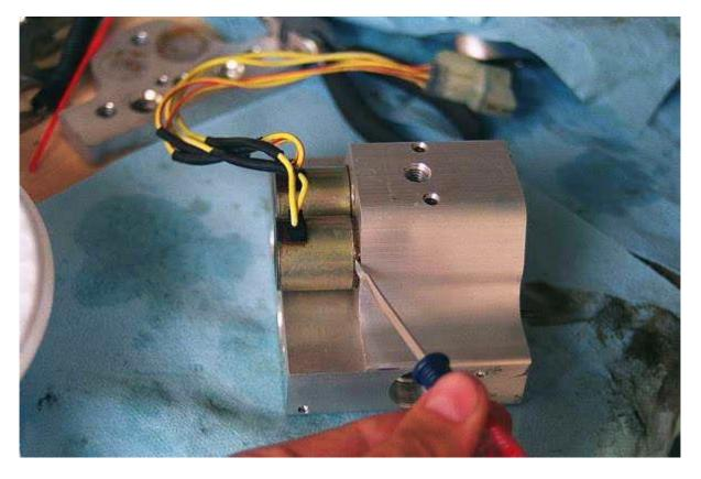
8) Remove the springs and spools behind the solenoid valves--pay close attention to the orientation of the spool as you remove it--you may have to turn the housing upside down and let them slide out. Once removed, look inside the spool and you'll see the tiny orifice. If this gets plugged, the system is hosed--that's why almost any gunk or particles cause such a mess.
