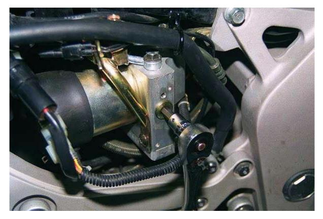
4) Push out return pumps from the inside where the motor mounted.
