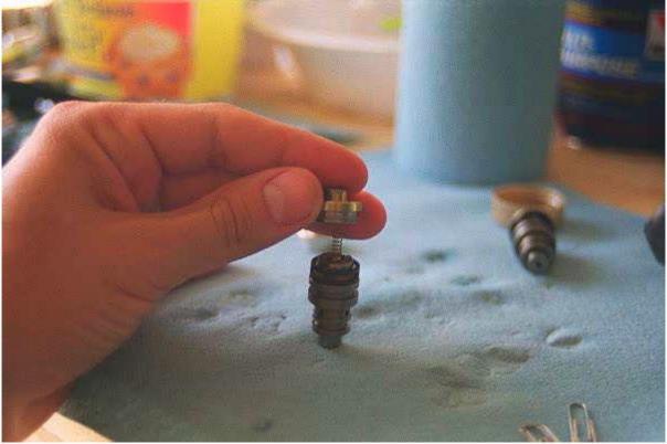
11) Break down all the other parts and clean, clean, clean. Be careful using brake cleaner as it may attack the o-rings--I used WD-40. Use the bronze (steel) wool to scrub off as much corrosion as you can from the steel parts. You may use naval jelly or a Dremel tool, whatever. Spray clean all of the passageways in the housing.
