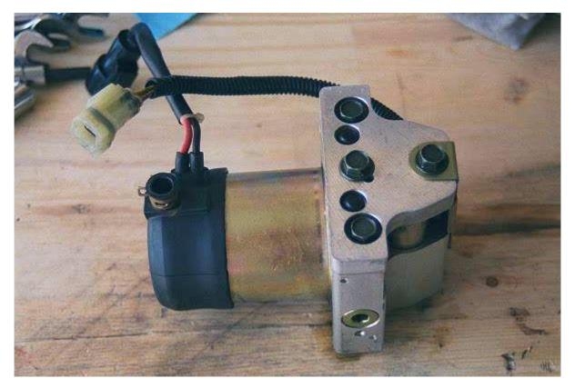
2) Remove electric motor. Move rubber cap--remove two long bolts
