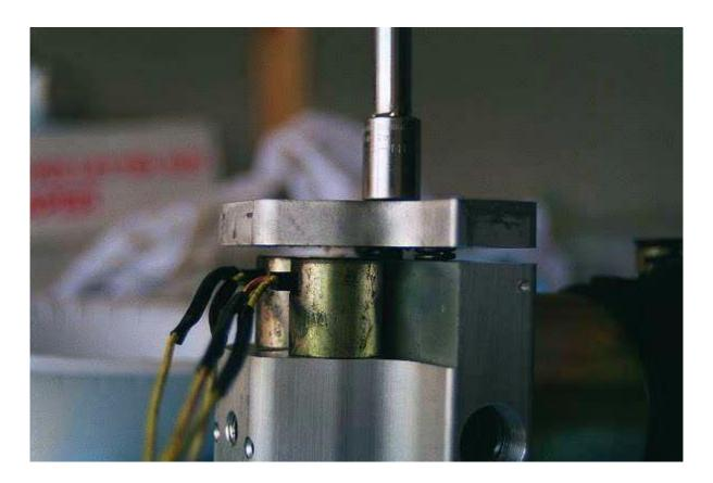
6) Remove the buffer chamber pistons. This can be a real pain--I was able to work a finger inside and "pull" the piston out.
