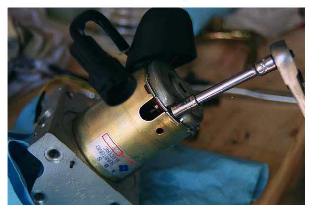
3) Remove 8mm hex nuts. Note: In the picture, I removed the plug while the HU was still in the bike. The next step is much easier to do with the HU on the bench.
